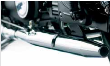
ACCESSORY MUFFLERS - SPEEDMASTER* For off road use only. Requires specific engine tune download.
