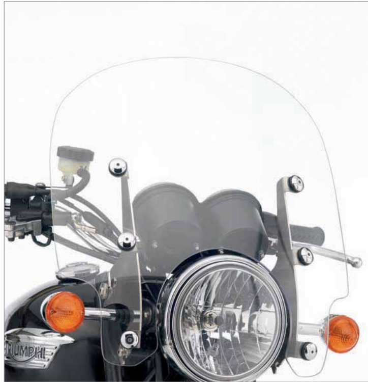
QUICK RELEASE SUMMER SCREEN Fits Bonneville & Bonneville SE Models. Height 10.63" from top of headlamp. Can be installed with lock kit A9700761.
